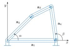
Fig. 2.1. System of four rods of Problem 2.3
